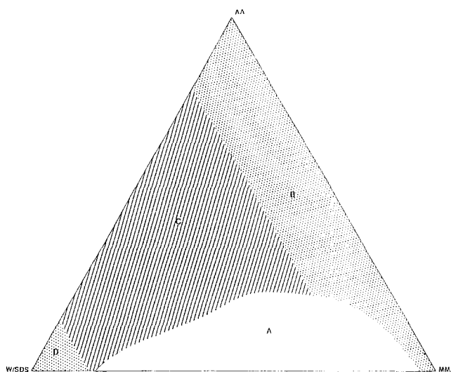
Figure 3 Phase-behaviour diagram for the system, methyl methacrylate (MMA), acrylic acid (AA), 20 wt% solution of sodium dodecylsulfate in water (W/SDS) and ethyleneglycol dimethacrylate (EGDMA) at 25°C. Compositions are on wt% basis and EGDMA is 8% of the combined weight of MMA and AA. Domain A: two-phase region, domain B: W/O Winsor-IV, domain C: bicontinuous Winsor-IV, domain D: O/W Winsor-IV
